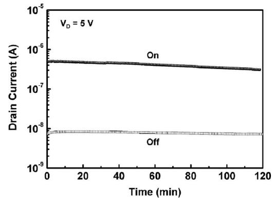
FIG. 4. Data retention properties of the on and off states of the FeFET under a floating gate ( $V_G = 0$  V,  $V_D = 5$  V) condition.
