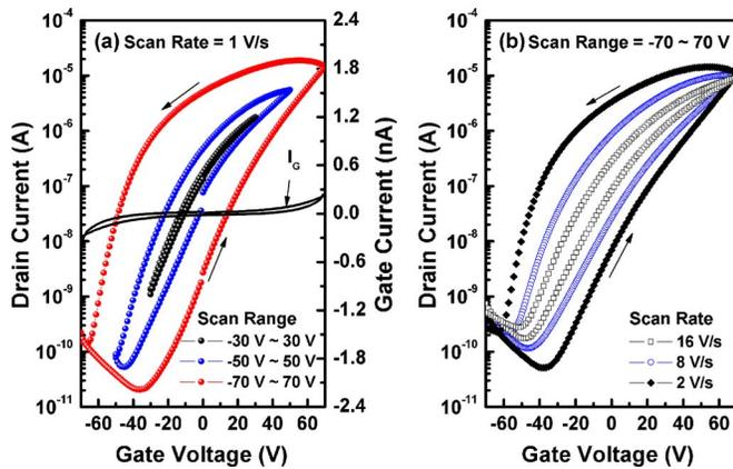
FIG. 3. (Color online)  $I_D$ - $V_G$  transfer characteristics of our FeFETs with (a) various scan ranges ( $V_G = \pm 30$ – $\pm 70$  V) and with (b) various scan rates (2–16 V/s).  $I_G$ - $V_G$  curve for the gate leakage level of our FeFET.
