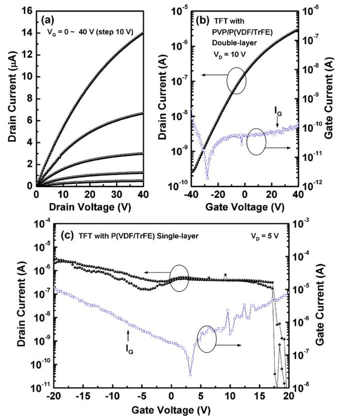
FIG. 2. (Color online) (a)  $I_D$ - $V_D$  output and (b)  $I_D$ - $V_G$  transfer characteristics obtained from the FeFET with PVP/P(VDF/TrFE) double layer in the pristine state. (c)  $I_D$ - $V_G$  transfer characteristics of the device with single P(VDF/TrFE) layer.
