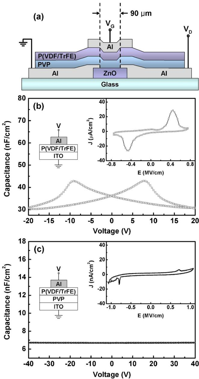
FIG. 1. (Color online) (a) Schematic cross section of our top-gate ZnO-FeFET with 450-nm-thick PVP/200-nm-thick P(VDF/TrFE) double insulator. (b) Capacitance-voltage ( $C$ - $V$ ) and the current density-electric field ( $J$ - $E$ ) (inset) characteristics of 200-nm-thick P(VDF/TrFE) single layer. (c) Capacitance-voltage ( $C$ - $V$ ) and the current density-electric field ( $J$ - $E$ ) (inset) characteristics of the PVP/P(VDF/TrFE) double layer.
