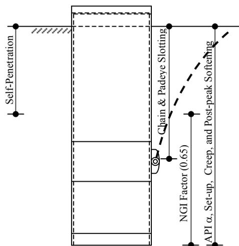
**Figure 5: Factors That Affect a Suction Pile's Axial Capacity**
