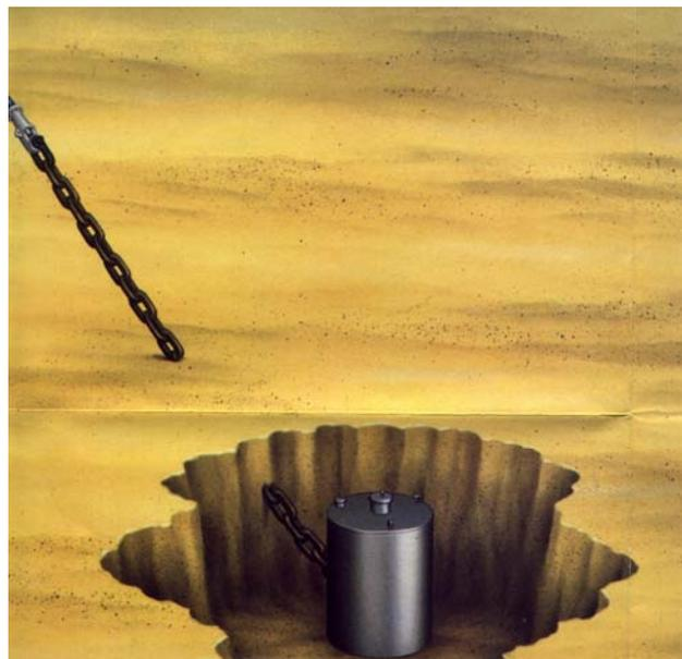
**Figure 4: A Suction Anchor Pile**
