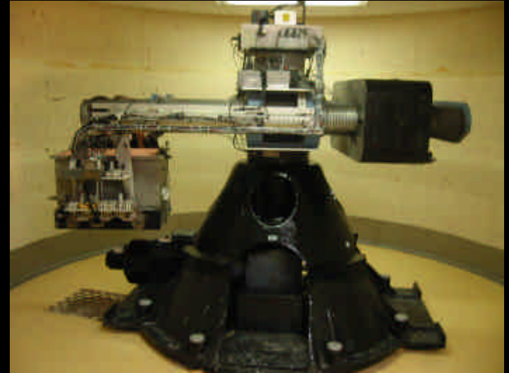
Beam centrifuge - 1.8 m diameter 200 kg capacity at 200 g
