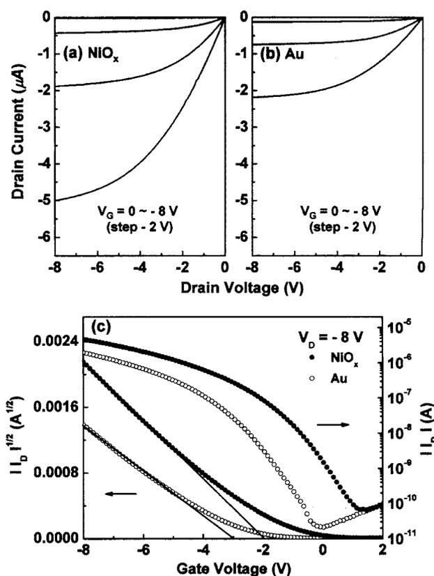
**Figure 3.**  $I_D$ - $V_D$  curves obtained from our pentacene-based TFTs with (a)  $\text{NiO}_x$  and (b) Au electrodes. (c)  $\sqrt{I_D}$ - $V_G$  and  $\log_{10}(I_D)$ - $V_G$  plots under a drain saturation condition ( $V_D = -8$  V).
