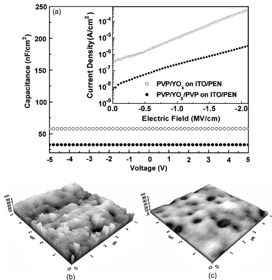
**Figure 2.** (a) Plots of C–V and (inset) J–E characteristics measured from Au-pad/dielectric insulator/ITO/PEN substrate structures. Chosen dielectrics were PVP (45 nm)/YO<sub>x</sub> (50 nm) and PVP (45 nm)/YO<sub>x</sub> (50 nm)/PVP (45 nm). (b) AFM images of ITO film coated on PEN substrate and (c) PVP (45 nm) layer spin-coated on ITO/PEN substrate.
