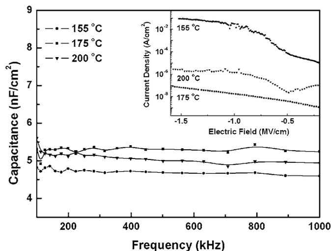
**Figure 1.** Plots of  $C$ - $f$  and  $J$ - $E$  (inset) characteristics measured from the 300- $\mu\text{m}$ -diam Au/650-nm-thick PVP/heavily doped  $p^+$ -Si structures.
