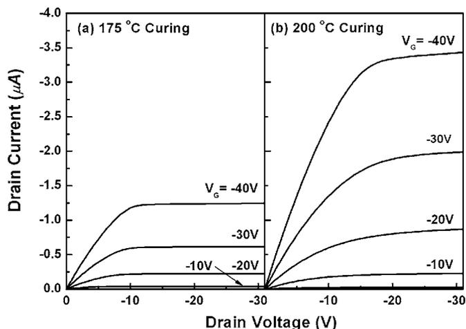
**Figure 2.** Drain current-voltage ( $I_D$ - $V_D$ ) curves obtained (after ten-times-repeated voltage sweep) from our OTFTs fabricated with PVP gate films cured at (a) 175 and (b) 200°C.
