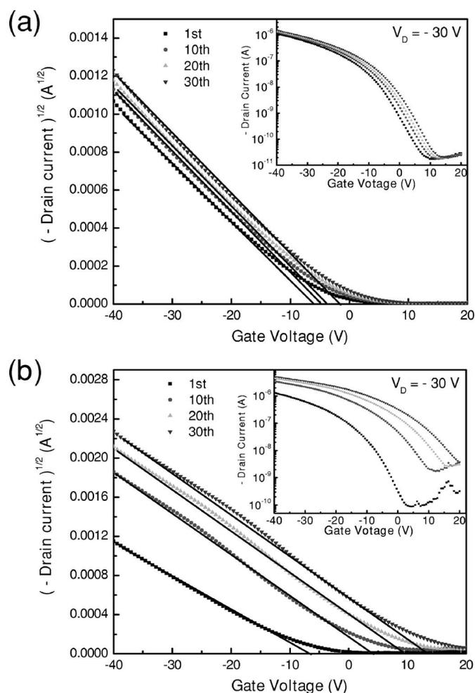
**Figure 4.**  $\sqrt{-I_D} - V_G$  and  $\log_{10}(-I_D) - V_G$  (inset) plots obtained with repetitive gate voltage sweep (up to 30 times) from our OTFTs fabricated using PVP gate films cured at (a) 175 and (b) 200°C.
