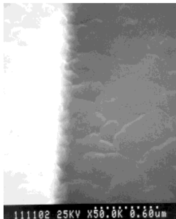
Fig. 10. SEM image of a pentacene thin film grown on \text{SiO}_2 and a Au electrode covered with a SAM of 1-hexadecane thiol. A similar grain size on both the \text{SiO}_2 and the Au/SAM surface is observed. The pentacene grain size transition region at the Au edge is eliminated. Reprinted from [84].
