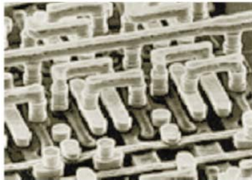
Fig. 2. Interconnect array, three metallization levels [3].
