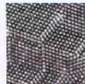
Atoms of silicon spacing ~tenths of nm
