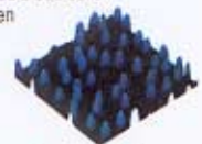
Quantum dot array -- germanium dots on silicon
